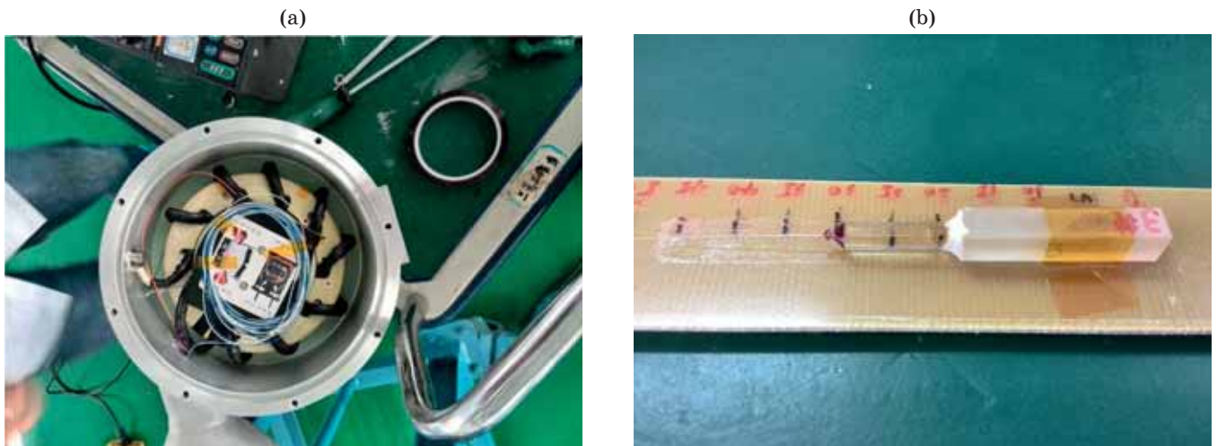
Fig. 5. Photos of the AF-FU-FOCT sensing head (a) and the MOC-FU-FOCT sensing head (b)
