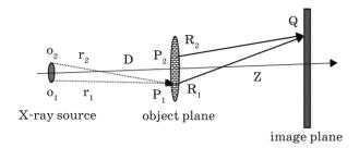
Fig. 1. Micro focus X-ray phase contrast imaging system diagram.
