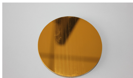
Fig. 11. Low-stepped mirror coated with gold reflector.
