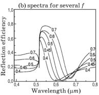
Fig. 4. Reflection efficiencies as functions of wavelengths and filling factors for p-polarizations and  $d = 0.12 \, \mu m$ .
