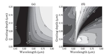
Fig. 2. Contour plots of reflection efficiencies for s-polarized (a) and p-polarized (b) lights when wavelength and grating depth are changed and gray scales are linear in efficiencies.
