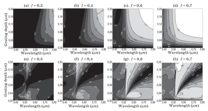
Fig. 3. Contour plots of reflection efficiencies for s-polarized (first lines) and p-polarized (second lines) incident lights as functions of wavelengths and grating depths at different filling factors: f = 0.3, 0.4, 0.6, and 0.7, respectively.
