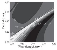
Fig. 5. Effects of grating periods on reflection resonances for  $d = 0.12 \mu m$ .
