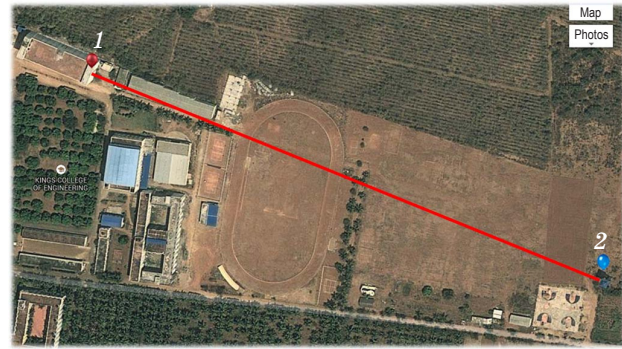
Fig. 1. Bird view (EOS) of optical propagation path for atmospheric C_n^2 field data measurement. The receiver system is located on the building at the left (1) and the transmitter system is located on the tower at the right (2).
